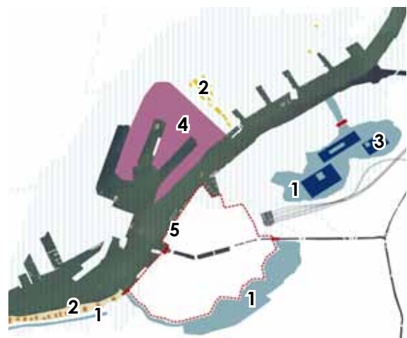
Creating space for water (1), buildings on stilts or with sacrificial ground floors (2), buildings on floating islands (3), raised ground level (4), flood defence structure around the city-within-the-moat (5).
